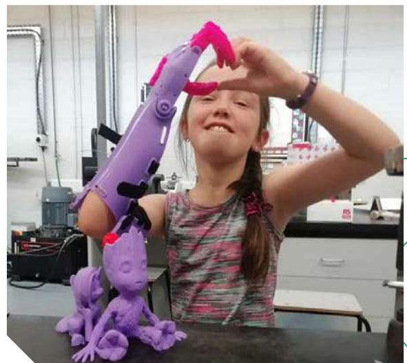
3D Assist manufactured prosthetics bio-plastic arm
